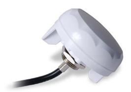
RV-19 is the integration of a high performance GPS patch antenna and a low noise amplifier into a low profile, extremely compact and fully waterproof enclosure. When connected to a GPS receiver with 2.5~3.3V DC antenna power, RV-19 provides excellent signal amplification and out-of-band rejection for that receiver.
