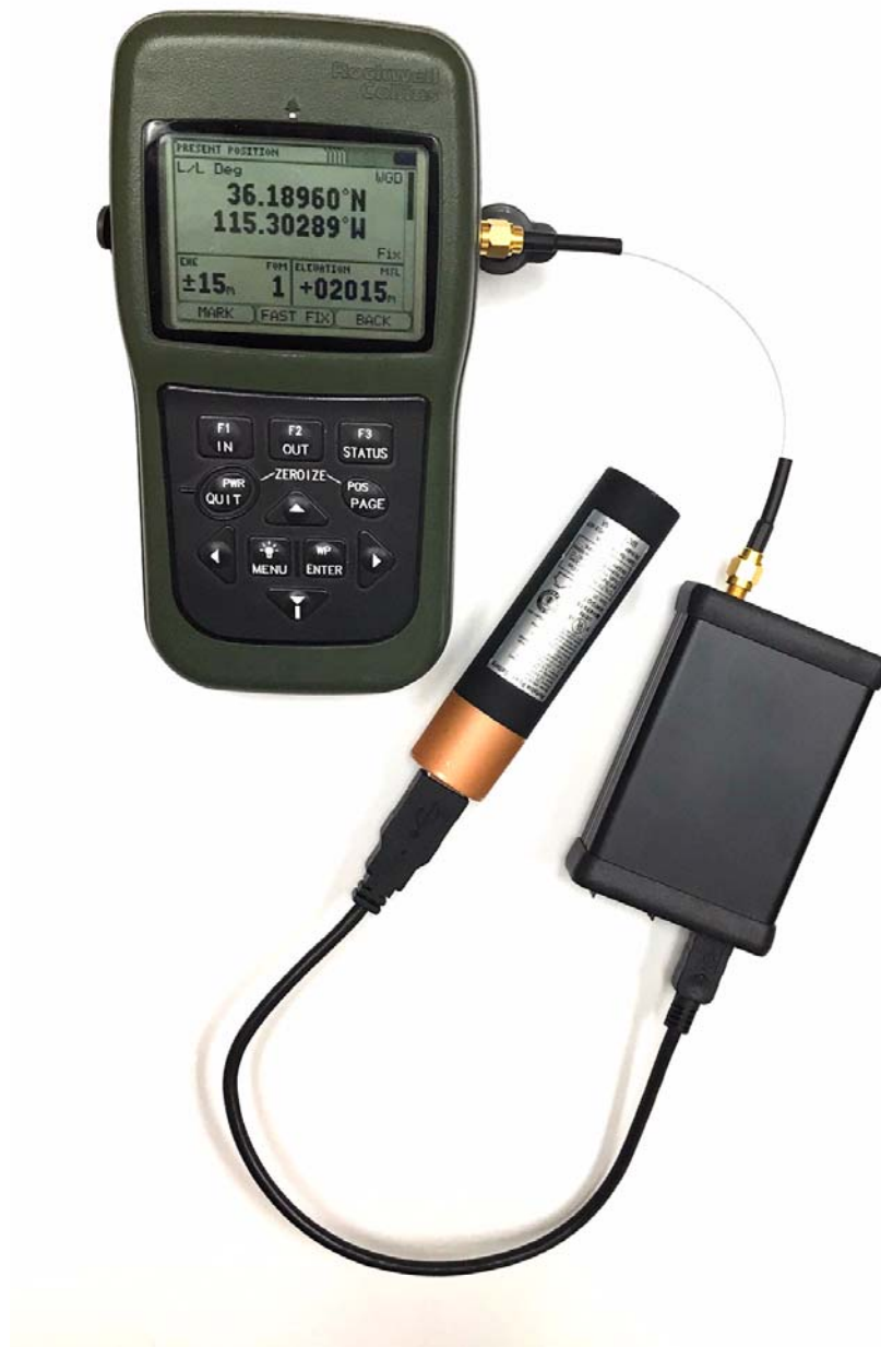
Figure 2.2 DAGR Target Receiver with Battery Operation of CLAW GNSS Simulator™
