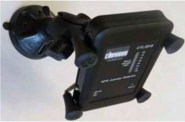
CTL3510 on optional universal mount with suction base
