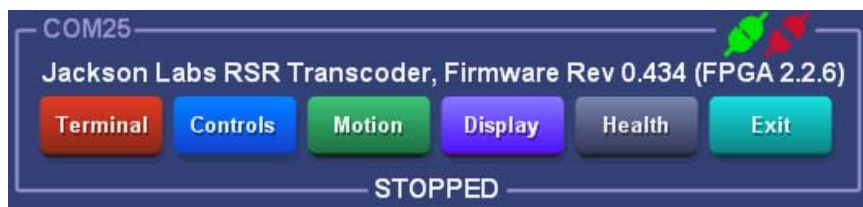
Figure 4.2 Connection header. Two USB devices are present, with an active connection to the RSR Transcoder at COM25
