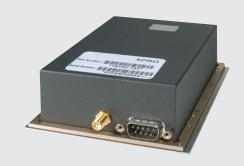
The XPRO is designed for long operating periods without maintenance (long-life rubidium lamp and extended crystal control range). With a  $5.0 \times 10^{-11}$  per month aging, the oscillator will maintain  $1.0 \times 10^{-9}$  frequency accuracy for 10 years or longer without recalibration.
