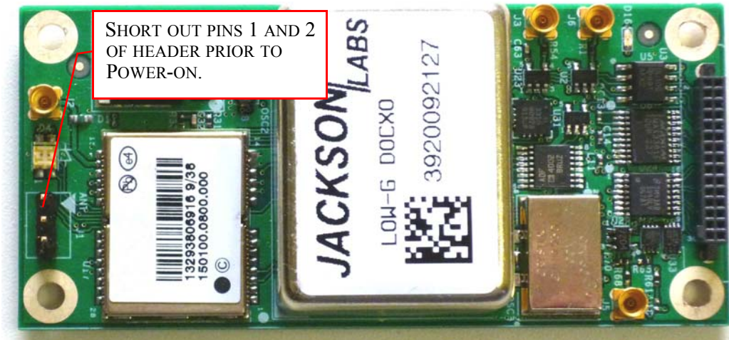
Figure 4.1 Location of J1 header
