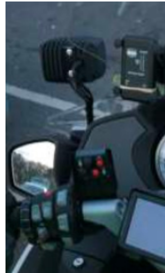
Close up of Jamming Detector on Motorbike
