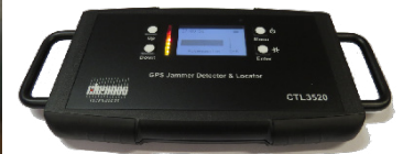
CTL3520 handheld GPS jamming detector with direction finding capability
