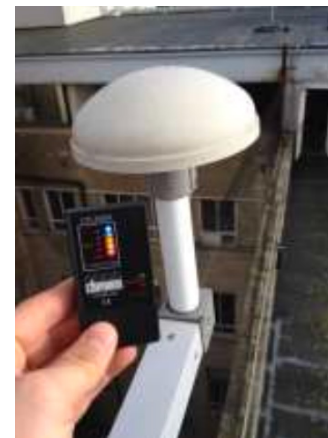
CTL3500 handheld GPS jamming detector
