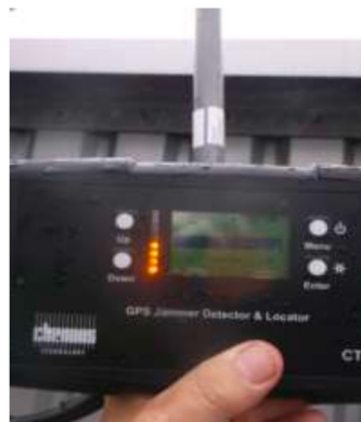
CTL3520 identifying Rogue Antenna at LD4
