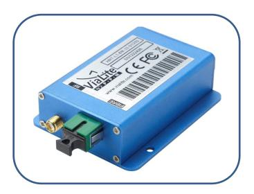
The **Blue OEM Link** is a small compact RF over fiber module which is available in *ViaLiteHD* RF bands up to 6 GHz, in either transmitter or receiver formats. The link is available with SC/APC or FC/APC optical connectors and SMA RF connectors.
