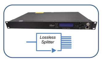
The *ViaLiteHD* Multizone Distribution Lossless Splitter allows for multiple receive points to be supplied by one transmitter with zero optical loss. It can be used with any *ViaLiteHD* RF over fiber frequency band, but is typically used in any fan-out application in satcom or timing applications, such as GPS or 10 MHz reference. The lossless splitter utilizes the low loss 1550 nm wavelength or any of the ITU DWDM channels for longer distances.
