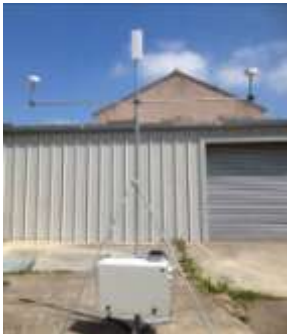
Figure 39: Field Deployed Sensor in Weatherproof enclosure
