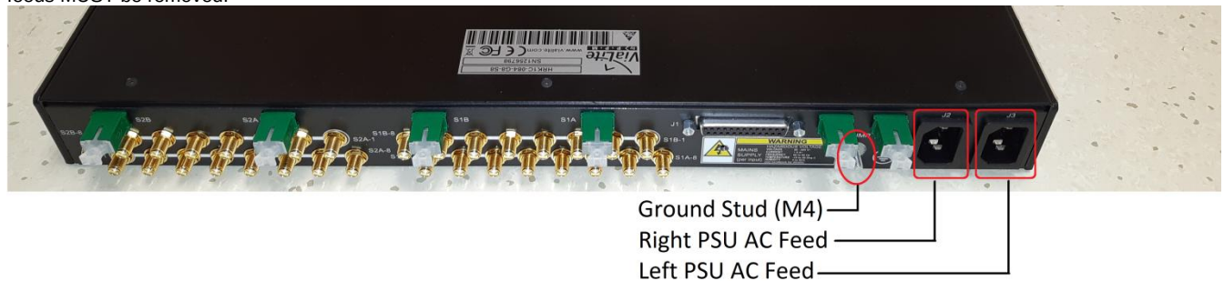
Electrical power connection locations for AC chassis
